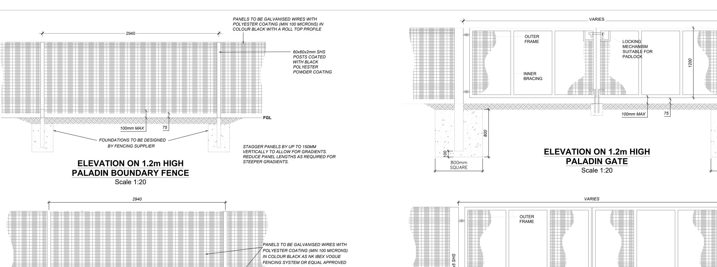
60x60x2mm SHS POSTS COATED WITH BLACK POLYESTER POWDER COATING AS NK IBEX VOGUE FENCING SYSTEM OR EQUAL FOUNDATIONS TO BE DESIGNED **APPROVED** BY FENCING SUPPLIER 2.4m HIGH PALADIN FENCE DETAIL 1:20
